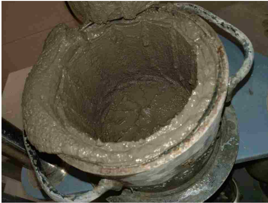
Figure 4-16 Discarded sample of a sample in pure plug flow due to high yield stress. This measurement was on the sand portion that passes sieve #50 at 42.5% of volume fraction.
